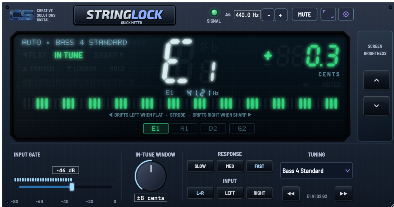
Strobe mode: near-zero deviation with illuminated green segments
